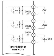
2 pulse input method(CW direction rotation pulse input) 1 pulse input method(Operating command pulse input) Note) If the power for driving pulse from external is over than +5V, please connect resistor
